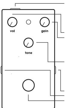
Power - Internal 9-volt battery or external DC 9 volt power supply is activated by plugging a cable into the input. The input cable should be removed when the unit is not in use to avoid running down the battery. If external DC 9 volt power supply is being used, unplugging the unit is not necessary.
